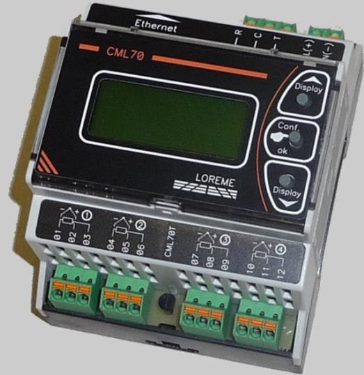
The CML70 is a four channels compact acquisition unit. Designed for demanding application in terms of accuracy and functional safety, the complete isolation of the product provide a total independence of each measurement channel.
